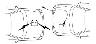
4. Remove the jumper cable from the positive (+) terminal of the disabled vehicle's battery.
